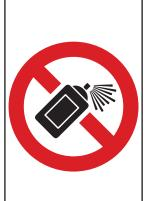
Never use aerosolpropelled sprays near the face port of the helmet or Band-Mask. The propellant used in these aerosols can invisibly damage the face port and cause it to shatter upon impact from any strong blow. If the face port fails underwater. the helmet will flood and drowning may result.
